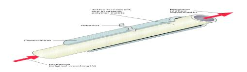
Fig 7 Odorant optical-fiber sensors
