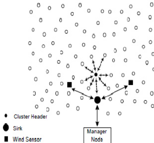
Figure4: A WSN for real-time forest fire detection [5].
